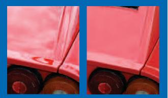
Gloss can also be a measure of the quality of the surface, for instance a drop in the gloss of a coated surface may indicate problems with its cure, leading to other failures such as poor adhesion or lack of protection for the coated surface.
